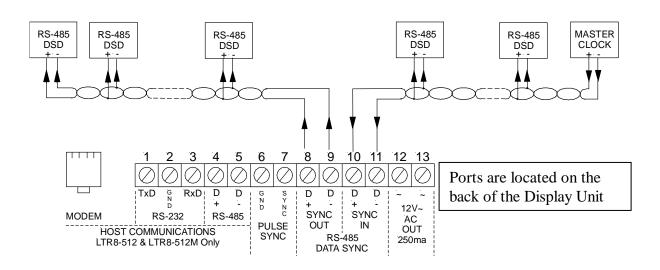
Note: Since the Sync In port can send as well as receive, 30 extra devices can connect here. If you already have a Master Source, such as an LTR-0, connect it and its string of clocks to the Sync In port, for a total of up to 60 devices.
